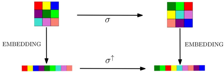
Although discrete, the embedding of a set of images  $\{f_i\}$  generated by the application of a group of permutations  $\Sigma$  lies close to a **smooth geometric structure** in  $\mathbb{R}^{m \times m}$ , whose nature may be useful in several computer vision problems.
